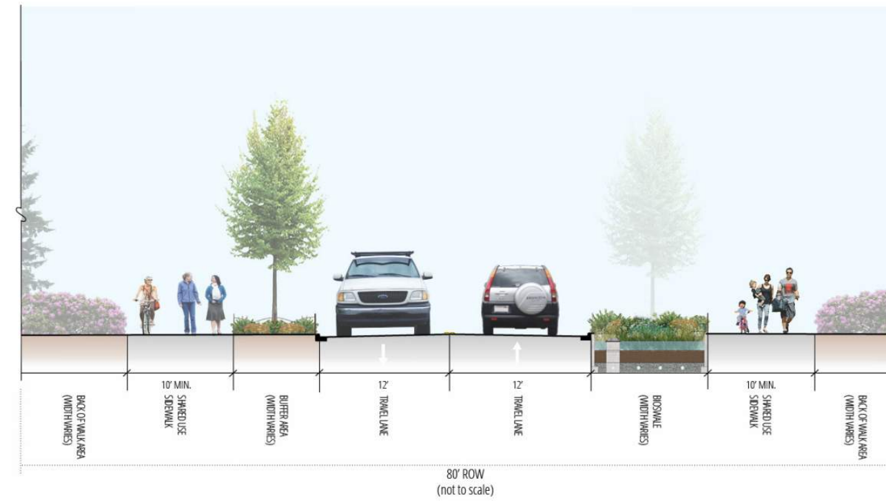
Section C with Bioretention Swale (looking east)
