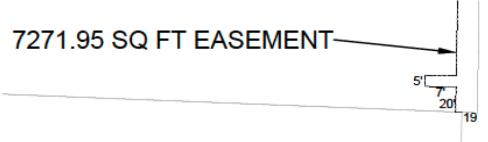
PROPOSED EASEMENT AREA AMENDMENT WITH ADDITIONAL 5'X27' FOR A TOTAL OF 5'X34' EASEMENT FOR ANCHOR
