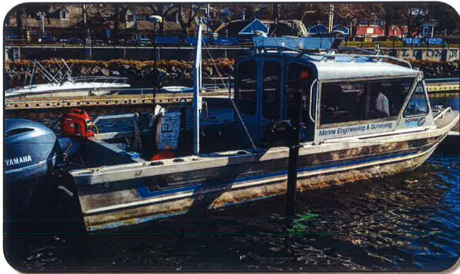
Figure 3. SHI's 24' aluminum survey vessel with MBES on side pole-mount.
