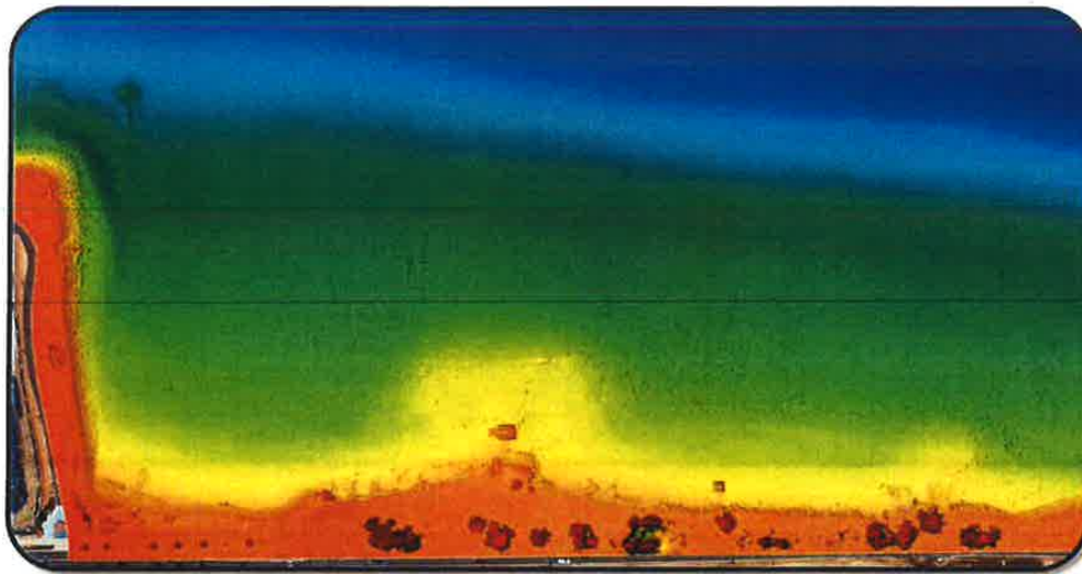
Figure 2. Combined MBES and sUAV survey at Point Ruston in 2019 illustrating high-resolution, shallow water imaging capabilities, shoreline measurement capabilities, and ability to identify underwater debris and hazards.
