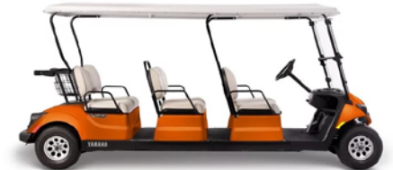
ICON i80 8 passenger, lithium-ion battery-powered golf cart
